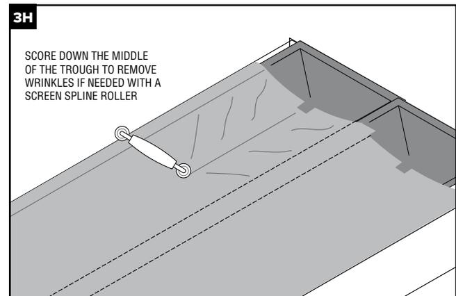
NOTE: In extreme temperature swings, trough material will expand and contract. Some wrinkling is acceptable but should not impede the flow of water.
