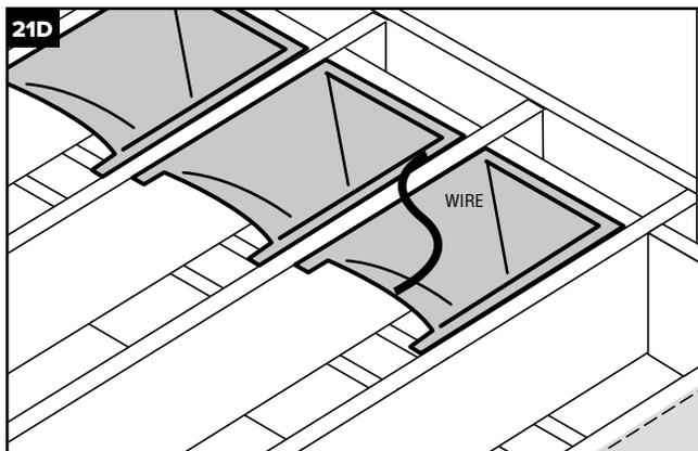
»Fish wire up through the gap between the trough and downspout. (21D)
