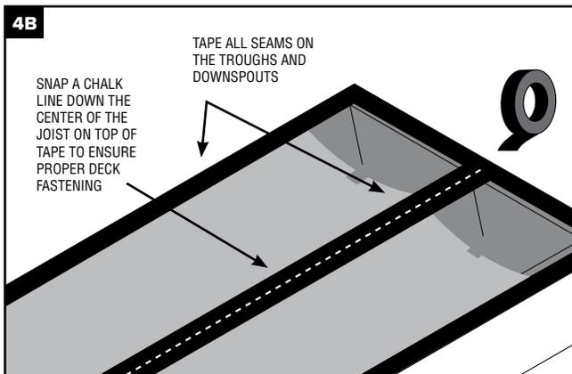
NOTE: *The butyl tape should never be put directly on wood. The trough material or a downspout must be below it.*
