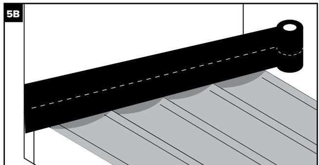
»Fold the Trex Seal Ledger Tape in half. Remove one of the release liners. Press to seal against the vertical surface at the 5-1/2" line. (5C)
